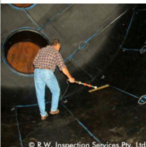
**ISOTEST® Test kit: Rubber lining incl. ISOTEST® inspect pro**
