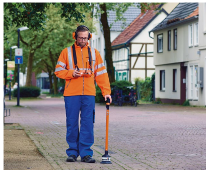
Pinpointing with the SeCorrPhon AC 200
