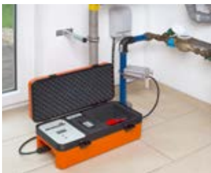
Locating metallic pipes and plastic pipes
