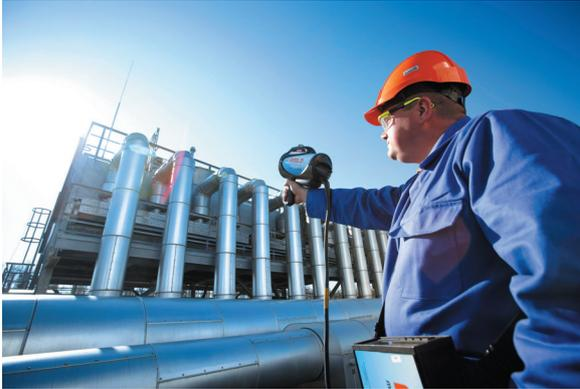
Revolutionary laser technique to check for gas leaks from a distance of up to 30 m
